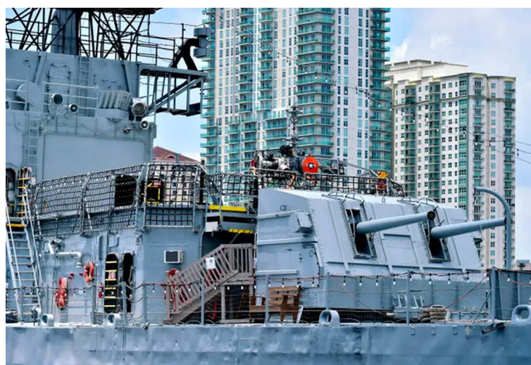
Among the Orleck's features is its 5-inch, 38-caliber gun turret on the ship's stern (Florida Times-Union)
