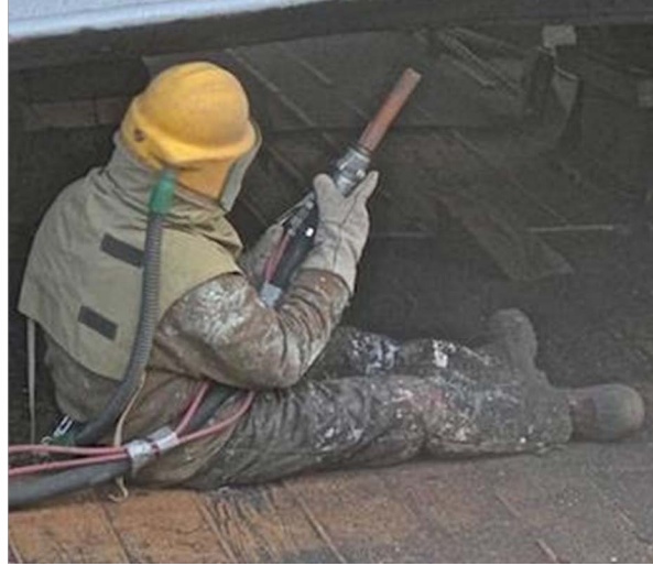
A shipyard worker media-blasts LV-112's hull during the 2012 dry-docking to prepare the hull for a survey and protective coatings, which will be required again during the upcoming haul-out for maintenance (U.S. Lightship Museum Photo)
