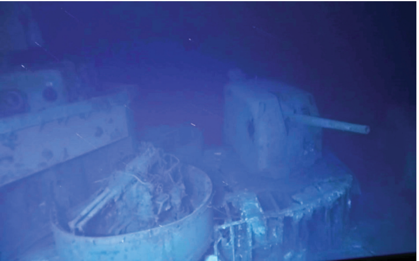
The forward starboard quarter of the Johnston's superstructure. Mount 41 is seen closest to the camera, Mount 52 to the right. Mount 52 was disabled by a shell fired by a Japanese destroyer at a shallow angle. According to Johnston's after-action report, this happened at approximately 0910, an hour before the ship sank. The entry hole is seen at the forward starboard corner of the mount, right at the trainer's seat. The trainer would have been killed instantly. The shell evidently hit the main body of the 5-inch gun and deflected downward before exploding, blowing out the rear port corner of the mount. One man was blown out of the forward port access door, which is seen missing. All 11 men inside Mount 52 were killed, and the mount remains frozen in that fatal instant. Credit: Caladan Oceanic, with permission
