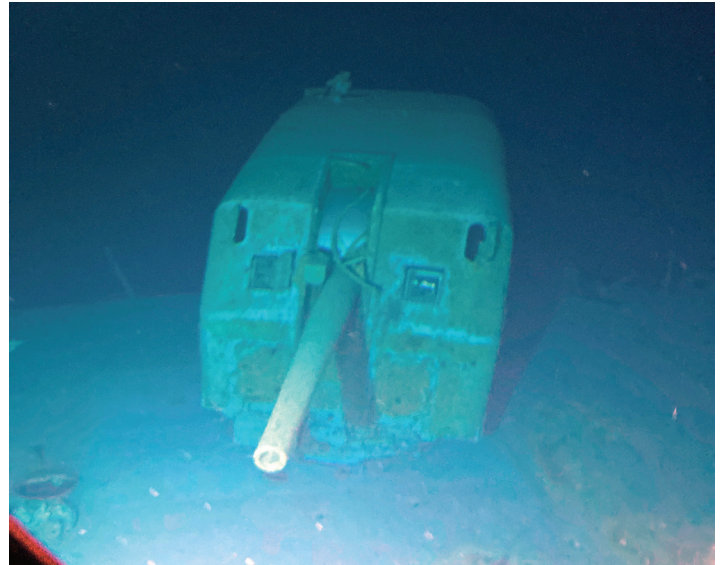
Mount 51, the farthest-forward 5”/38 gun mount on Johnston's fore deck. The gun is trained to starboard, but was disabled by a shell from the Japanese cruiser Suzuya approximately 1 hour before Johnston sank. Credit: Parks Stephenson
