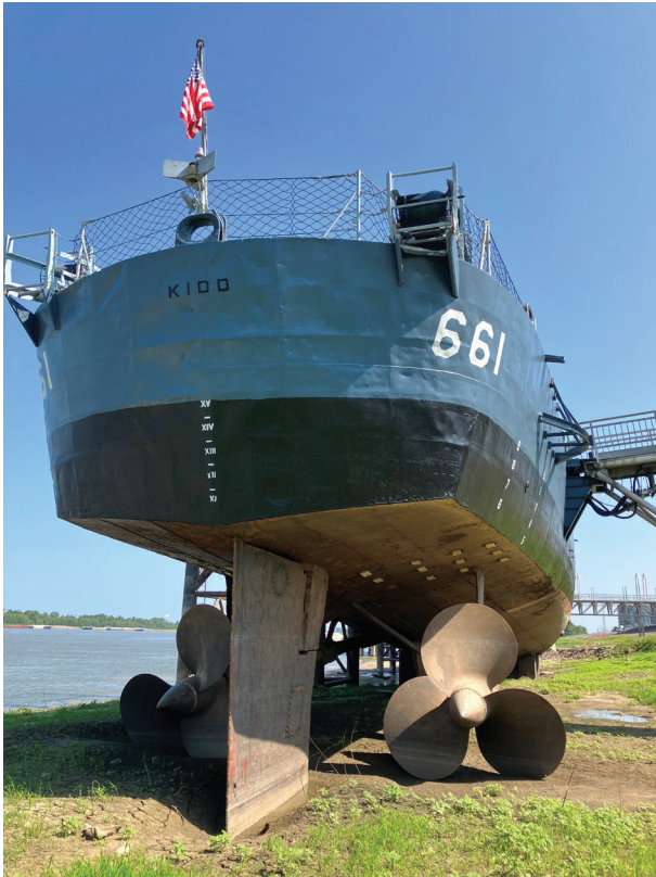
Left: Stern view of USS Kidd (DD-661) during low river levels. This view highlights her rudder and twin-screw arrangement, a rare view for a museum ship. USS Kidd is the only museum ship that is displayed and open to visitors regularly both in and out of water. Credit: Parks Stephenson
