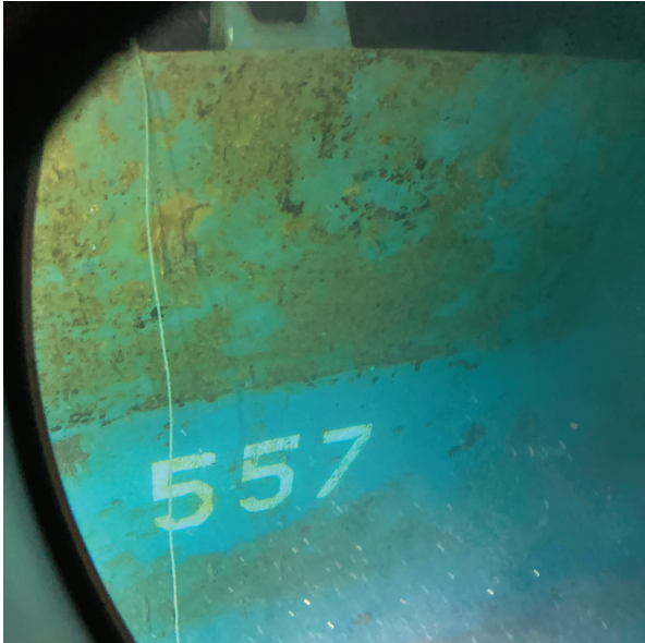
Close-up of the hull number painted on Johnston's starboard bow. There was not much corrosion in areas that were left untouched by the fires of battle. Credit: Parks Stephenson
