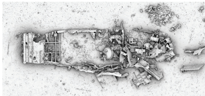
Two-dimensional site plan of a Japanese Daihatsu landing craft based on a 3D photogrammetric model. This landing craft rests on the seafloor off Saipan at a depth of 10 meters (32 feet). Site plans are used to monitor site degradation over time.
