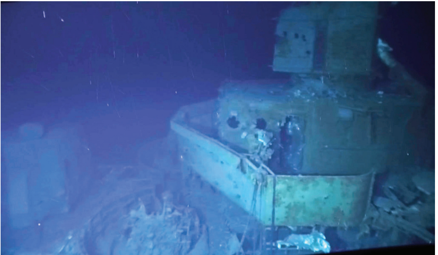
Port side view of the superstructure, showing the bridge wing and the burned and destroyed Mount 42 (forward port dual 40-mm mount). Credit: Caladan Oceanic, with permission.
