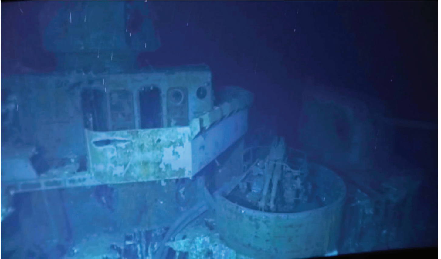
Starboard side bridge wing, showing the undamaged Mount 41 (forward starboard dual 40-mm mount). Evans did not want the pilot house closed off while he moved back and forth, even those were Condition Zed fittings. The hooked-open doors can be seen in the dive imagery. Credit: Caladan Oceanic, with permission.
