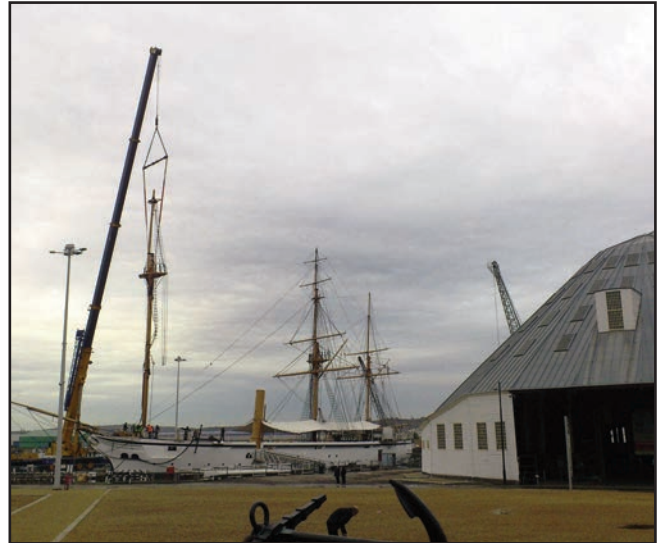
Above: A large crane is used in stepping the new mast on HMS Gannet, the sole surviving sloop of Queen Victoria's Royal Navy.
