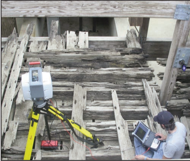
Above: Paul Davidson (HABS), scanning Cairo's boiler deck. Photograph courtesy National Park Service.
