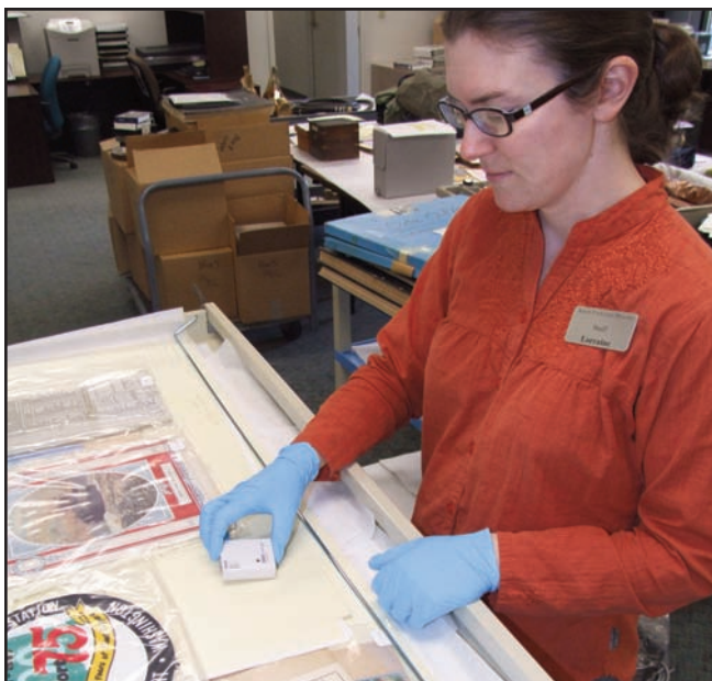
Above: Ms. Lorraine Scott places a HOBO data logger in a map drawer to determine temperature/RH differences within enclosed storage cabinetry.
