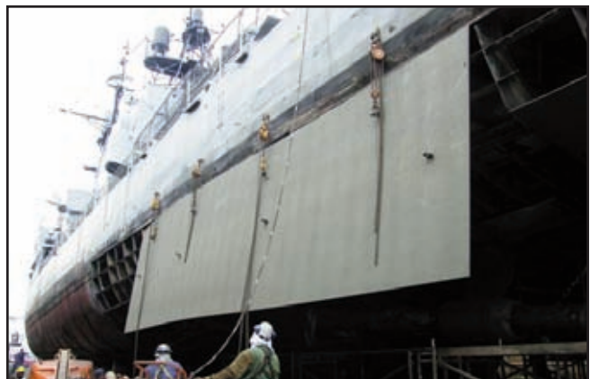
Below: "On with the new..." Brand new steel plating is placed over the exposed frames of the Laffey.
