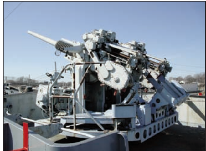
Above: One of the twin 3”/50 caliber gun mounts onboard the Salem. It is believed that she is the only historic ship museum to have twin 3”/50s. Photo by Jason Hall
