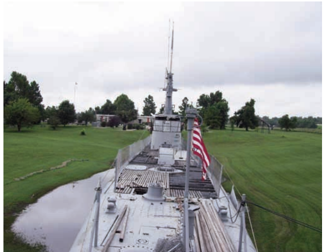
Above: The major concerns for the ship are clearly seen in this image: the slight list, standing water around the hull, and the desperately needed deck replacement.
