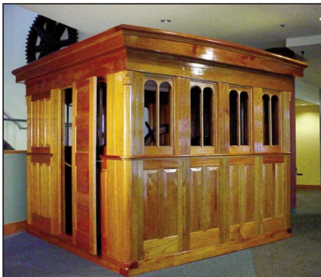
Above: Built in Independence Seaport Museum’s own boatshop, the beautifully-recreated pilothouse currently stands in the Museum’s lobby. It will be installed aboard OLYMPIA in the project’s next phase. Photo courtesy Independence Seaport Museum.
